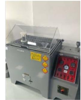
Salt spray test chamber
